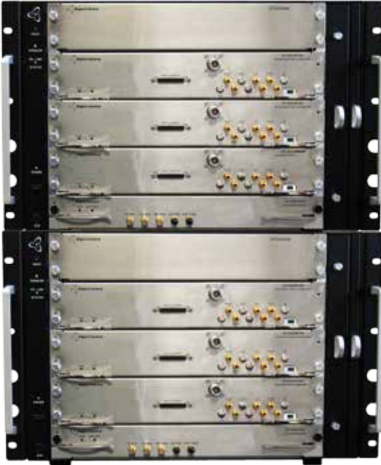
Example Configuration - two Giga-tronics Advanced Signal Generation and Analysis Systems containing RF Signal Generators, RF Upconverters, RF Downconverters, Arbitrary Waveform Generators and Digitizers all in a self-contained AXIe standard chassis
