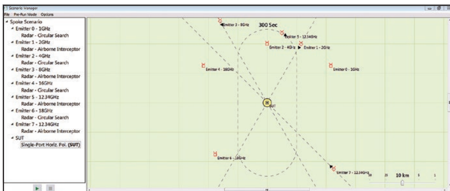
FIGURE 3 – The TEmS battlespace is simulated using a 500 km x 500 km, flat earth environment. Pulse descriptor words from every emitter are calculated in real-time for 10 ns timing resolution as the platforms move through battlespace.
